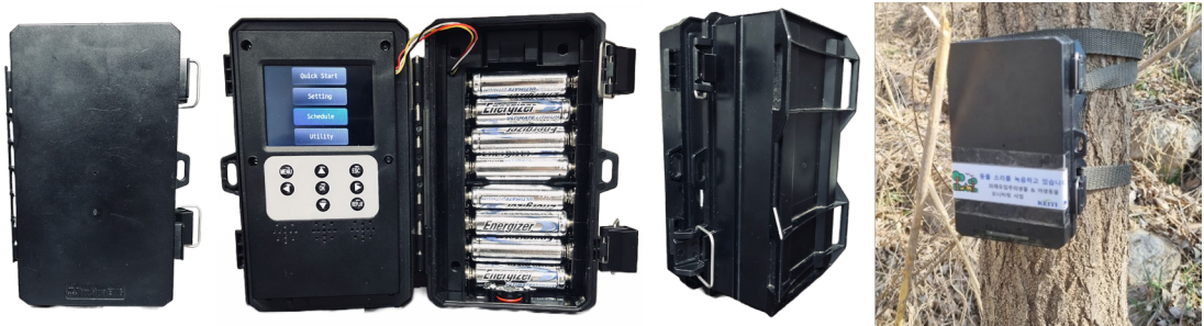
〈Fig. 2〉 Shinhwa Engineering's bioacoustic recording device used for frog species monitoring.
